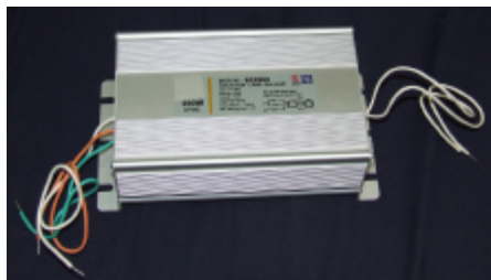
INDUCTION LAMP BALLAST
